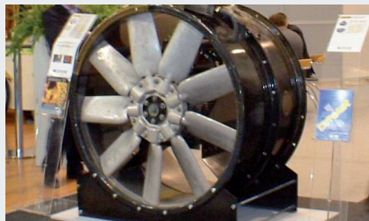
Axial duct fan CC-HT after high temperature testing at 400°C/2 hours according to EN 12101-3.
