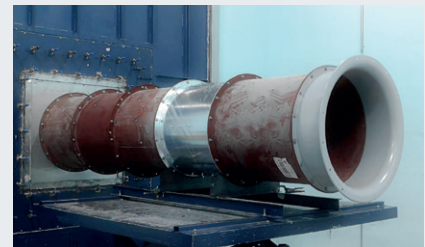
A TA fan being tested in AMCA.
